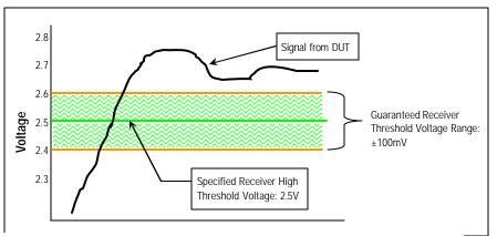
Figure 3 Receiver high threshold range
