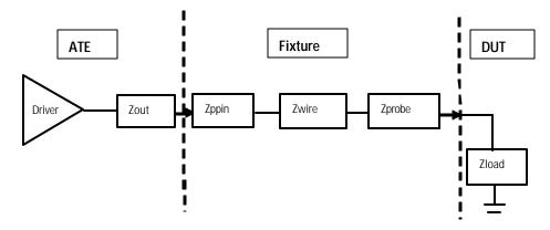
Figure 5 Impedances during digital testing
