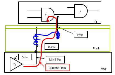
Figure 4 Current flow from the driver during backdriving
